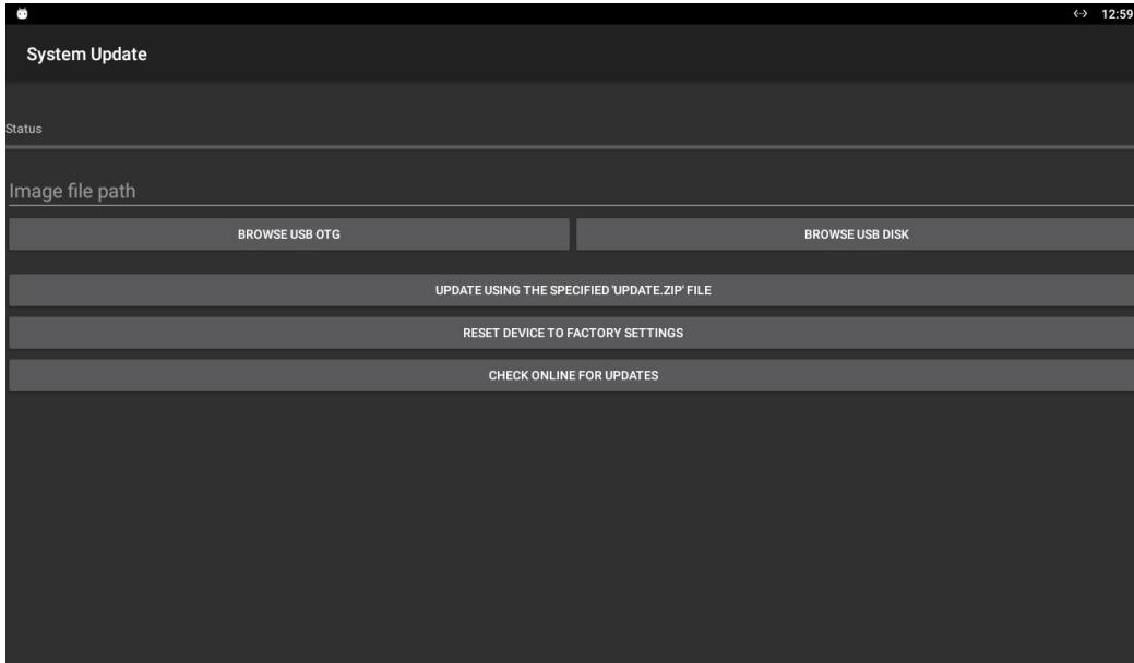
After starting this app, you can either update your DIVUS KNX IQ using a special file or you can reset the device to factory settings. By selecting the last option the device will automatically reboot, execute the reset and start with the factory defaults.
