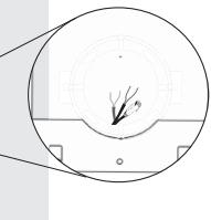
Fix the metal gasket with 4 countersunk screws (not part of the delivery)
