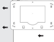
Place the metal gasket on the mounting box - make sure that it is horizontal. The 4 brackets look in your direction.
