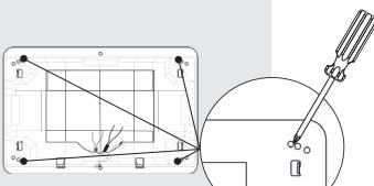
Fix the metal gasket with 4 countersunk screws (not part of the delivery)
