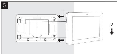
Insert the panel into the mounting brackets
