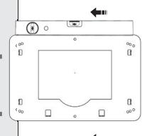
Place the metal gasket on the mounting box - make sure that it is horizontal. The 4 brackets look in your direction.
