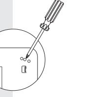
Fix the metal gasket with 4 countersunk screws (not part of the delivery)
