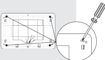
Fix the metal gasket with 4 countersunk screws (not part of the delivery)
